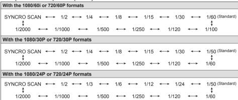
When [SYSTEM FREQ] is set to [50Hz]
