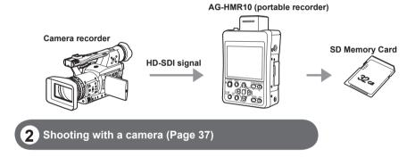
When the portable recorder is connected to the AG-HCK10G camera head (optional), data can be recorded onto an SD Memory Card.
