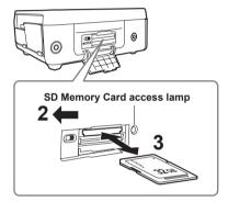
To insert: Insert the card with the label facing up, and push until it clicks firmly into place.
